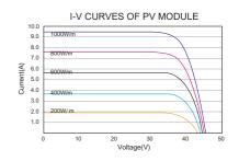
Percent of the indicated Values of Isc, Voc, and Pmax under Standard Test Conditions (Irradiance of  $1000W/m^2$ , AM 1.5 Spectrum and Cell Temperature of  $25^{\circ}C$ )
