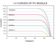
Percent of the indicated Values of Isc, Voc, and Pmax under Standard Test Conditions (Irradiance of 1000W/m², AM 1.5 Spectrum and Cell Temperature of 25°C)
