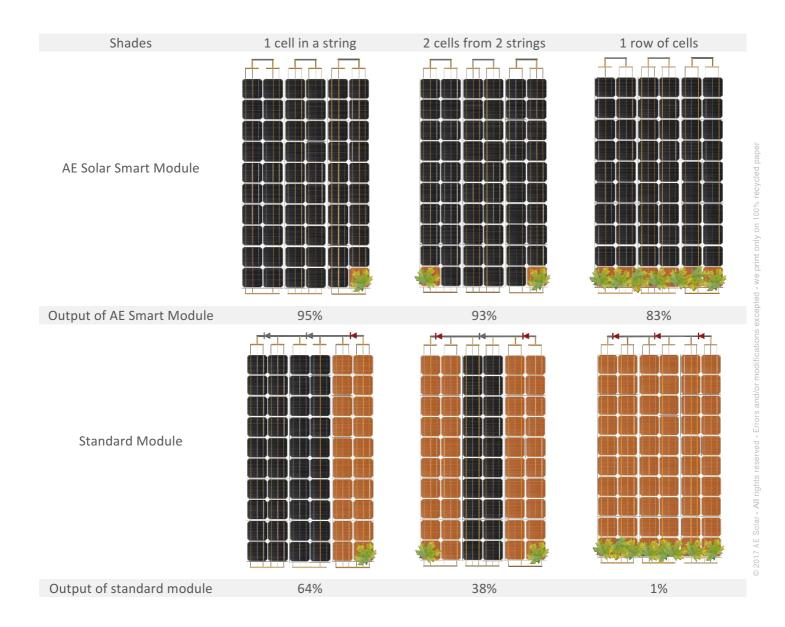
When multiple cells are in shade, a hot-spot free module can generate 80% more power, compared to a standard module.
