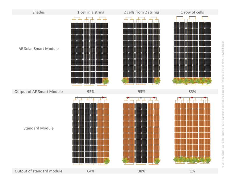
$When \ multiple \ cells \ are \ in \ shade, \ a \ hot-spot \ free \ module \ can \ generate \ up \ to \ 80\% \ more \ power, \ compared \ to \ a \ standard \ module.$
