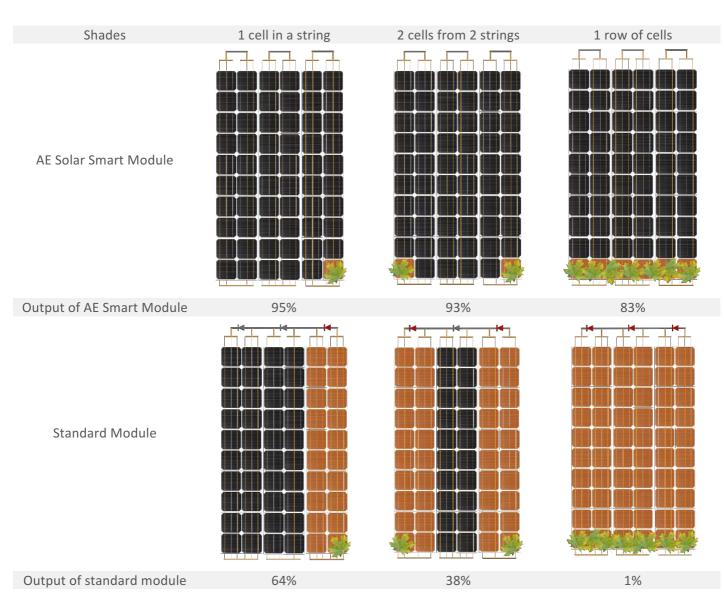
When multiple cells are in shade, a hot-spot free module can generate up to 80% more power, compared to a standard module.
