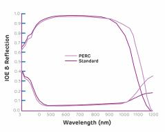
PERC technology enables better light capturing abilities at longer wavelength, weak and diffused light and in cloudy conditions.
