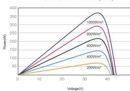
P-V CURVES OF PV MODULE(370W)
