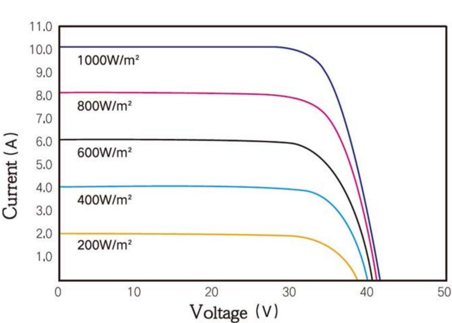
\*STC (Standard Test Condition): Irradiance 1000W/ m², Module Temperature 25°C, AM 1.5
