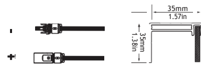
PV Connector Model - TT01, 1000V, 30A, IP67
