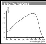
PPAM uses high efficiency solar cells with substantially higher spectral response at blue wavelenght and thin 3-bus-bar for best thermal properties.
