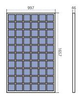
Rated values under Standard Test Conditions (STC: 1000 W/m², 25°C, spectrum AM 1,5)\*
