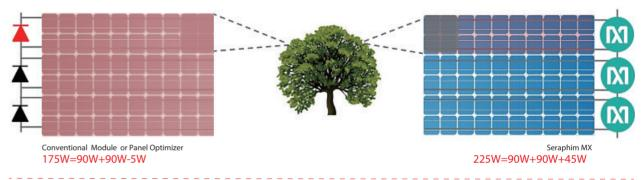
Seraphim MX reduces the shading effect significantly, prevents hot-spot formation, and eliminates diode failures. In the meantime, it will lower Operation and Maintenance costs.
