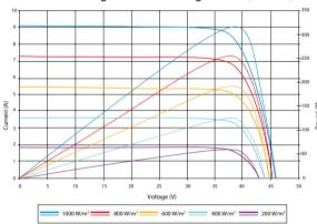
Excellent performance under weak light conditions: at an irradiation intensity of 200 W/m² (AM 1.5, 25 °C), **96.5%** or higher of the STC efficiency (1000 W/m<sup>2</sup>) is achieved
